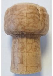
Check also that the closure is held high enough because elongation of the closure out of the jaws will generate lipping.
