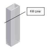
3. Fill the cell (3) with the required sample. Cell should be  $\frac{2}{3}$  full.
